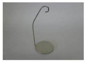
The DRY REVELATOR CONTROL DISC is metallic. Its diameter is 10 cm (4"). It allows the user to control under UV-A the pollution of the dry revelator. Fluorescents marks will indicate it.
